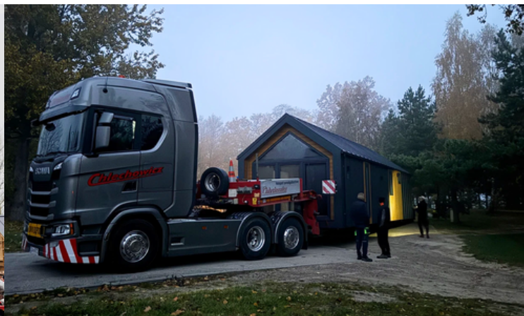
A lorry with a EURO low loader semi-trailer on which the house moves on the road
