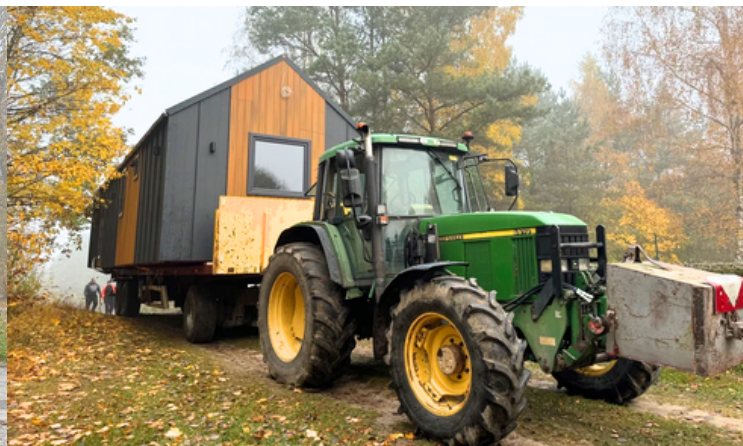
During this particular unloading, 2 tractors were needed to pull the trailer up a hill that could not be reached by a truck.
